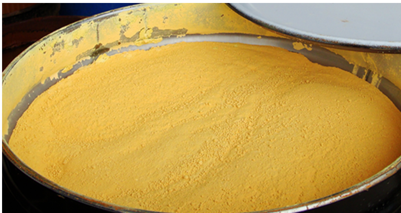
Uranium oxide "yellowcake" is processed from uranium ore before enrichment.
